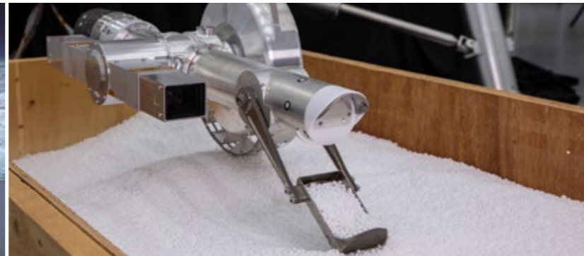
The PolyU-developed system accomplished the tasks of automatic sample collection and packaging on the lunar surface.
